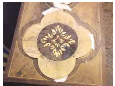
A Macassar ebony and pearwood piece of marquetry work ready to be glued in place
